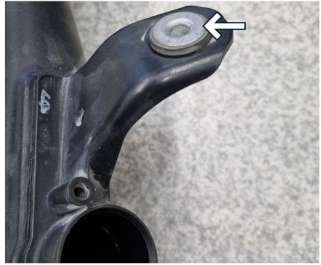
Located on the turbo there is a pin screw that needs to be removed. Unscrew it with a 3mm Allen key. If the Allen head is corroded tighten two M6 nuts hard against each other and then remove the pin screw with help of the outer nut.
