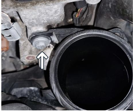
Remove the T25 Torx marked on the photo above and then remove the entire top half of the turbo inlet pipe.
