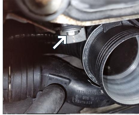
Install the included O-rings on the CNC aluminum joiner. Lubricate the O-rings with some WD-40 or similar. Then gently push the CNC joiner into the turbo compressor housing. Fasten it with the included M6 screw.
