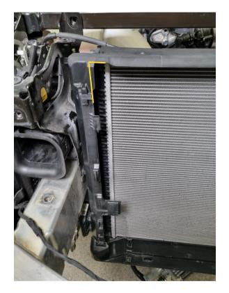
Note for step 11-18: It is possible to cut the plastic radiator supports with the front radiator air duct in place but it is a bit tight space. To have better access you can remove the front air duct by first removing the lower support beam (under bumper beam) then remove the radiator air duct.
