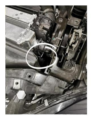
Now you can slide the radiator in from the top. Be aware of the oil cooler and main radiator and don't push down hard, carefully wiggle down in place.
