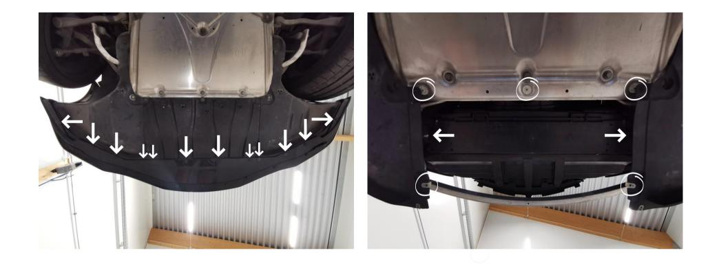
Remove the 12 x 8mm hex screws holding the bottom part of the bumper. Then preferably with the help of an assistant, remove the bumper. Start by pulling out the sides and disconnect the electrical connections on both sides, then pull the bumper forward to remove it from car.
