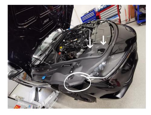
Remove the two plastic clips on each side holding the plastic panel over the hood latch.
