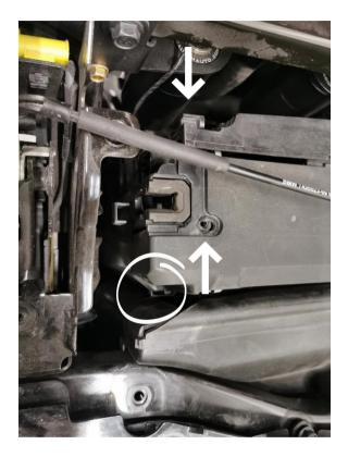
Remove the 4 x T30 screws holding the top plastic and fan to the radiator. Release the clip and lift up the fan a bit to remove the top plastic.
