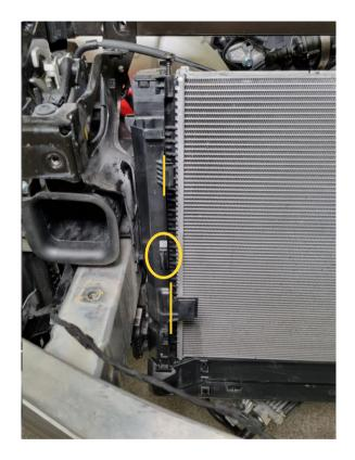
Cut the brackets according to lines in picture from the right plastic radiator support and cut the tab circled in picture flush.
