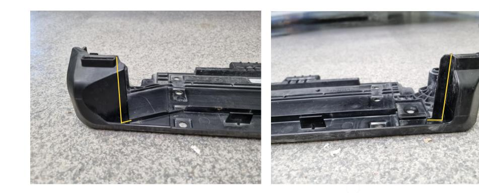
Cut the right side of the lower radiator support in a straight line down from the clip mount.
