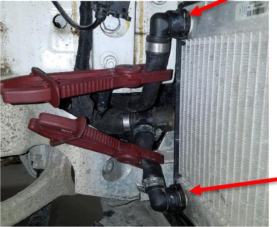
8. Remove the Torx T30 that's holding the radiator in its place. Gently remove the radiator from the vehicle. Empty the radiator from coolant in a clean bucket if you want to re-use the coolant.
