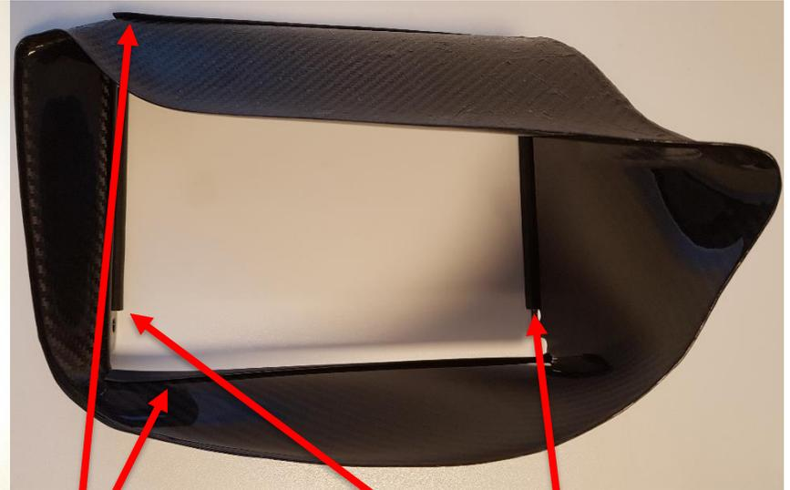
Cut the rubber edge sealing and apply on the top & bottom of the carbon fiber air guide.
