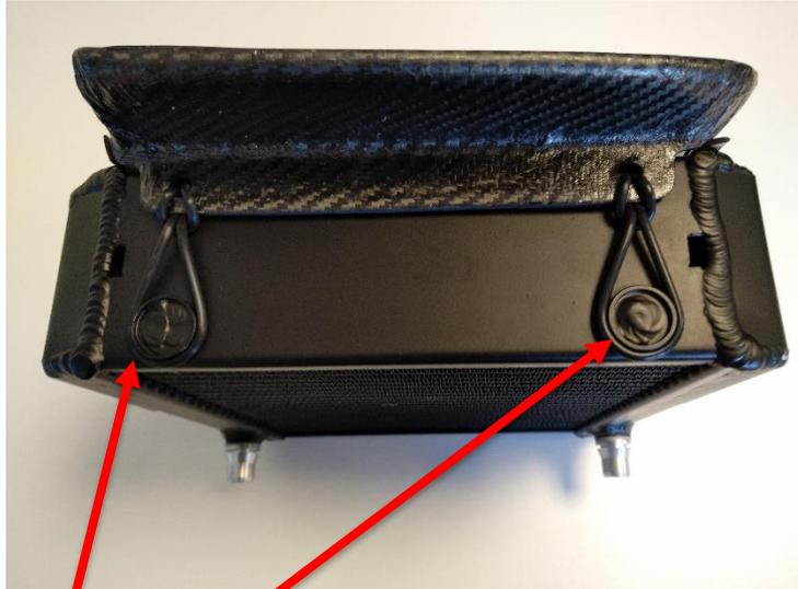
Thread the four rubber O-ring thru the holes on the air guide and make a loop, place it over the tab on the do88 radiator.
