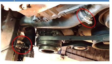
14. You may need to grind the plastic bracket slightly on the right-hand side. Keep in mind the radiators are hand build and deviation between units can occur.
