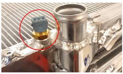
Now install the do88 radiator into your car. This can be done both from underneath (easiest) or from the top. To protect the new aluminum radiator during installation, put for example cardboard sheets over both sides of the core when putting it in place.
