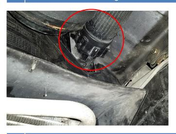
6. Remove the upper radiator hose (1x hose clamp & 1x metal clip) and also remove the bleeding hose (1x hose clamp & 1 plastic tab clips)
