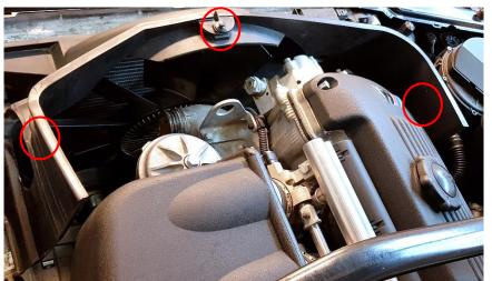
**8.** Disconnect relay and cable connector from the radiator fan cover.
