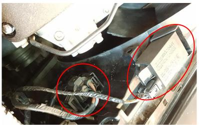
Remove the oil cooler from the radiator 2x Torx T25
