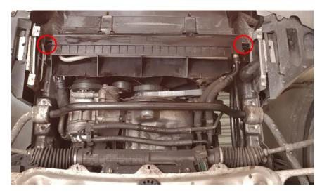
Remove the radiator fan. Loosen it with a 32mm open-end wrench. NOTE! It is left hand threaded. You need to keep the shaft fixed with a big flat end screw driver while loosing it. Lift the fan out of the car together with the fan cover.
