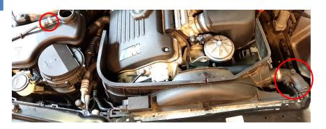
**7.** Remove the 3x plastic clips then remove the two radiator fan air guides.
