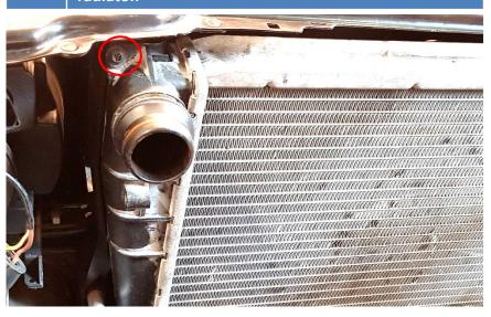
Now gently remove the radiator. You may take it up or downwards. After that remove the lower radiator hose 1x Hose clamp and 1x cable connector.
