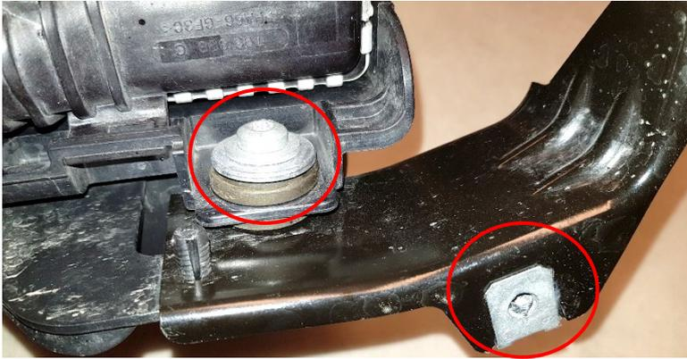
13. Install two of the rubber grommets and screw clip previously removed to the included bracket.
