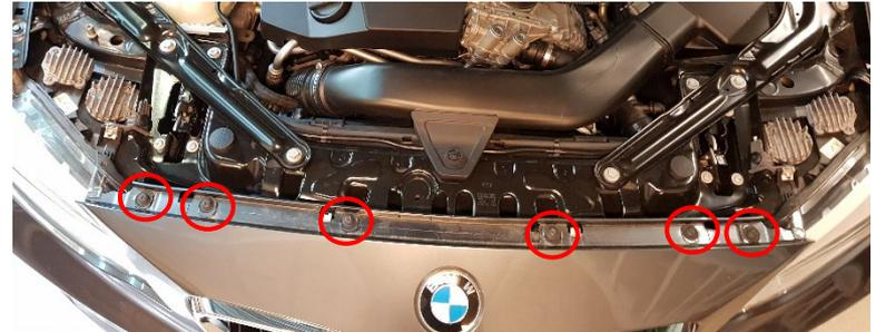
3. Remove the inner wheel arch on both sides, 7x Hex 8mm screws on both sides.
