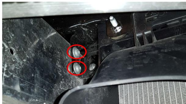
12. Remove 3x Torx T30 screws and 1x screw clip from the radiator support frame. Two of the rubber grommets and the screw clip will be reused.
