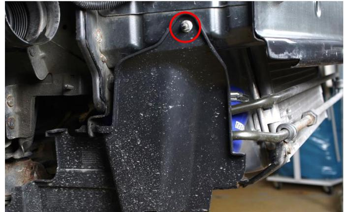
**11.** Remove the air guide from the top of the intercooler by pulling it upwards.
