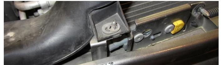
8. Disconnect the horn connector and cable clips. Also remove the 2x 10mm hex nuts holding the radiator support brackets.
