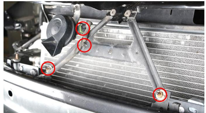
**9.** Remove the radiator support by removing 8pcs of 10mm (on facelift 6pcs) hex head screws.
