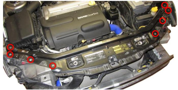
**10.** Remove the air guides positioned at each intercooler connection 2x Hex 10mm nuts.
