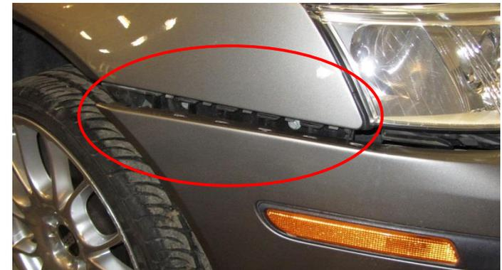
6. Remove the headlights by removing 3pcs of 10mm (on facelift 2pcs 10mm & 1pc 8mm) hex screws on each headlight and then pull/lift forward so you can disconnect the electrical connector from the headlight and then remove headlight from vehicle.
