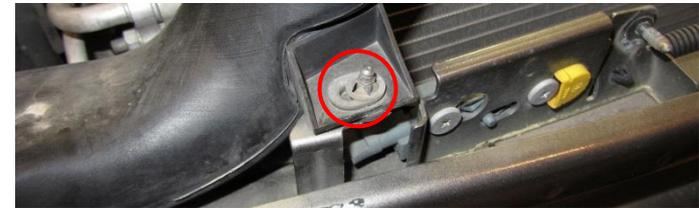
**11.** Remove the air guide (1.) from the top of the intercooler by pulling it upwards. Remove the 2pcs Torx T25 screws (2.) that attach the AC condenser to the intercooler.
