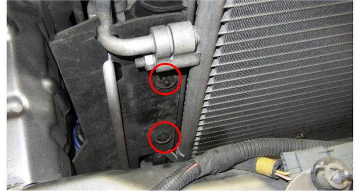
**13.** Lift the power steering cooling pipe up from its slots. Support the power steering pipe by hand and temporarily attach it to the bumper beam with zip tie or similar.
