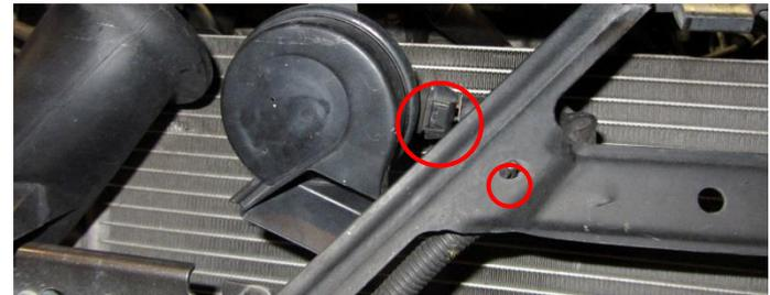
8. Remove the two Torx T25 screws that secures the air inlet pipe to the radiator support.
