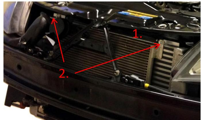
**12.** Remove the air guides on both sides of the intercooler by gentle pry out the tabs in the washer and then remove from intercooler pin. Remove air guides from intercooler.
