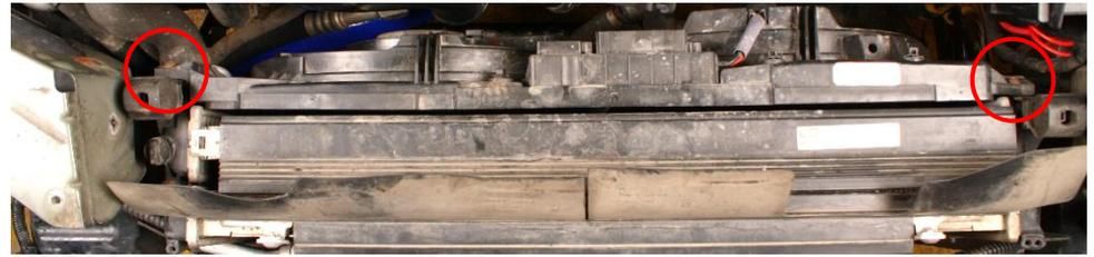
**23.** Now drain the radiator from all coolant, use the plastic drain screw in the lower right corner. The disconnect all three radiator hoses.
