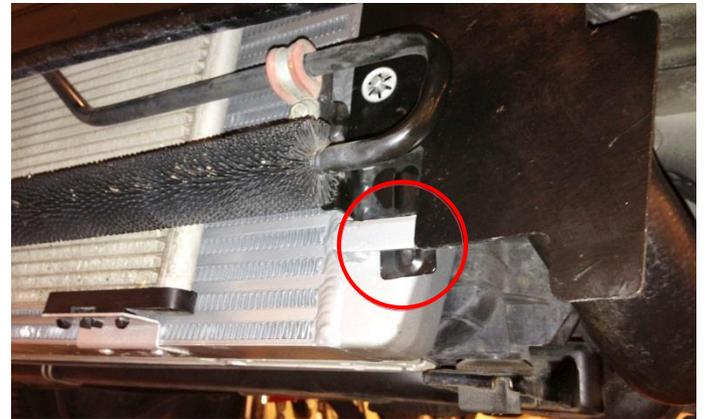
**14.** Lift the AC condenser upwards from its slots in the intercooler and tie it toward bumper beam as much forward as possible.
