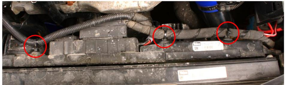
**22.** Remove 2x T25 Torx screws in top of each corner of the fan shroud.
