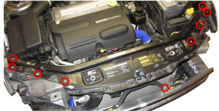
**10.** Remove the air inlet duct by screw up the washers, twist the pipe on its lower connection so it lifts from the attachment point then twist at the same time as you pull forward until it comes loose from the air box.
