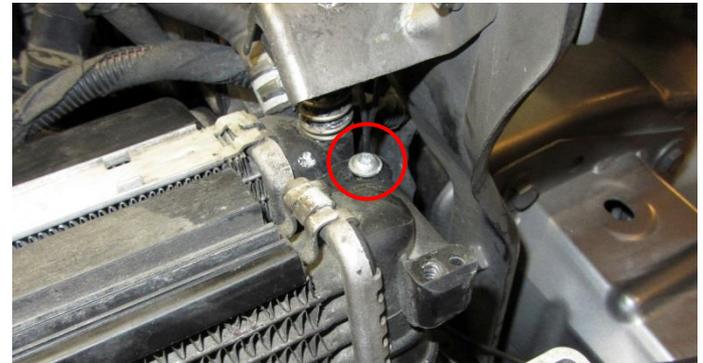
17. Remove the intercooler by lifting it up from the radiator slots and then carefully remove the intercooler downwards starting with the left hand side and then the rest of it according to picture.
