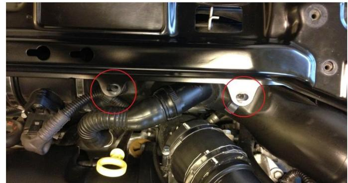
**9.** Remove the radiator support by removing 8pcs of 10mm (on facelift 6pcs) hex head screws on top of it and 2pcs of 10mm hex head screws in the bottom of the cross member.
