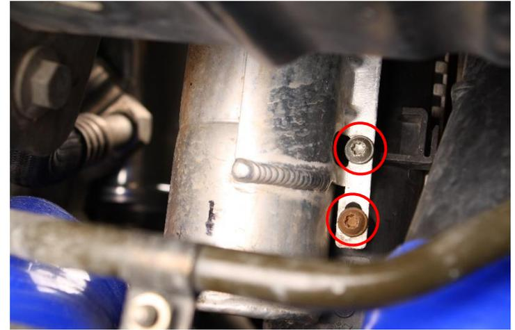
**24.** Remove 2x T25 Torx screws holding the air conditioning filter to the radiator.
