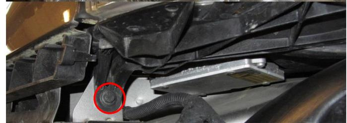
7. Disconnect the electrical connector from the horn and remove the cable clips from the front cross member.
