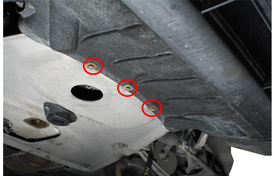
5. Remove the 4x Torx T30 on top of the bumper.
