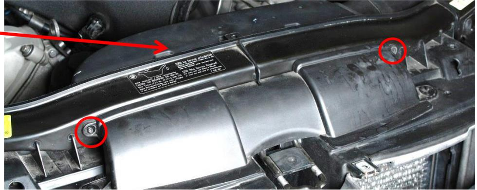
9. Remove 2x Hex 10mm and gently lift the entire air filter box straight up and remove it from vehicle.
