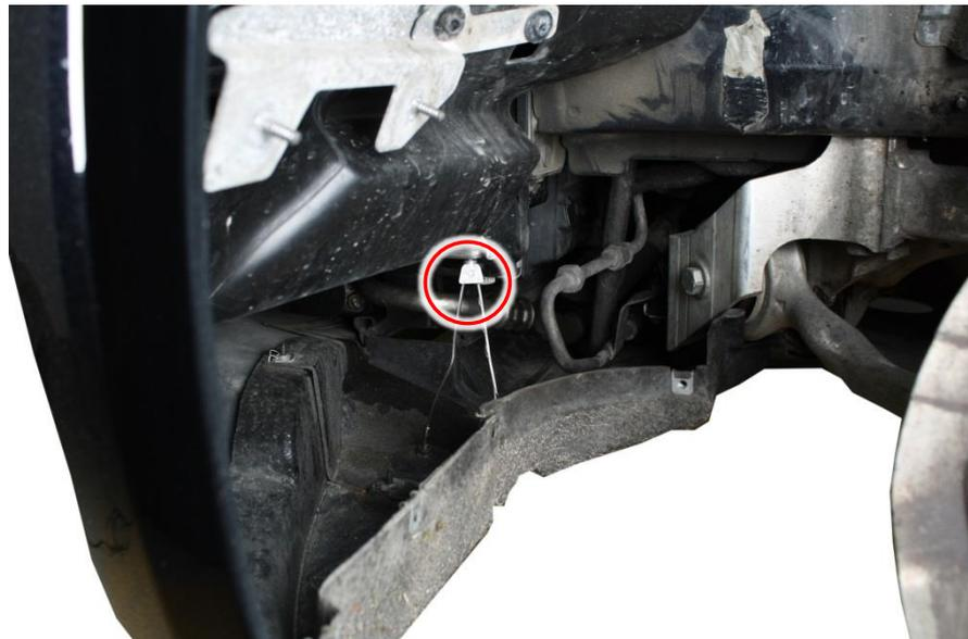
3. Remove 2x Hex 8mm in each upper corner of the bumper on both sides. (These become visible after you have removed the inner fenders).
