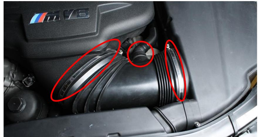
8. Remove 2x Torx T20 and pull out the fresh air duct to the air filter box.
