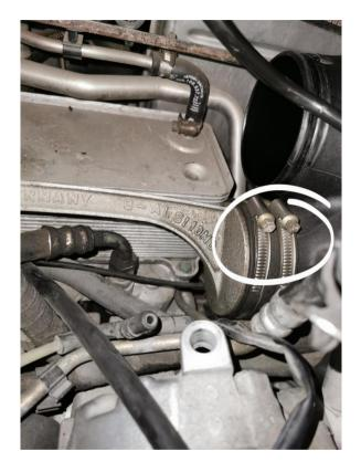
In preparation for the installation, you need to loosen the hose clamps holding the two intake manifolds together (2 on the left and 2 on the right). This is necessary to do because it might have to be rotated so it clears the plenum.
