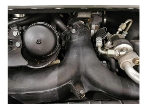
Disconnect the air mass meter electrical connector and loosen the airbox hose clamp. Then rotate the airbox counterclockwise to remove it from the car
