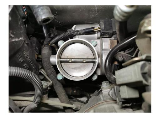
Now pull the charge pipe gently back until it loosens from the throttle body. Then disconnect the vacuum hose from the charge pipe before you remove it entirely.
