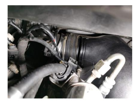
Remove the P-clip holding the AC-Accumulator. Then remove the bolt located on the back of the AC-Compressor 13mm Hex and the 10mm Hex under the Accumulator. Separate the pressure valve from the bracket. The hose connected to the bottom of the pressure valve needs to be disconnected and moved to the side to remove the plenum.
