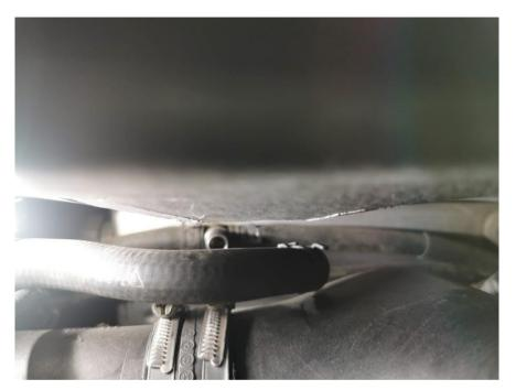
Disconnect the three vacuum lines to the left of the throttle body flange from the plenum. The vacuum line with the back pressure valve is preferably removed during installation, the other two is easily moved to the side to give space.
