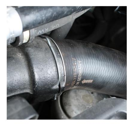
Disconnect the hoses from the charge pipe (y-pipe) they are retained by c-clips.
