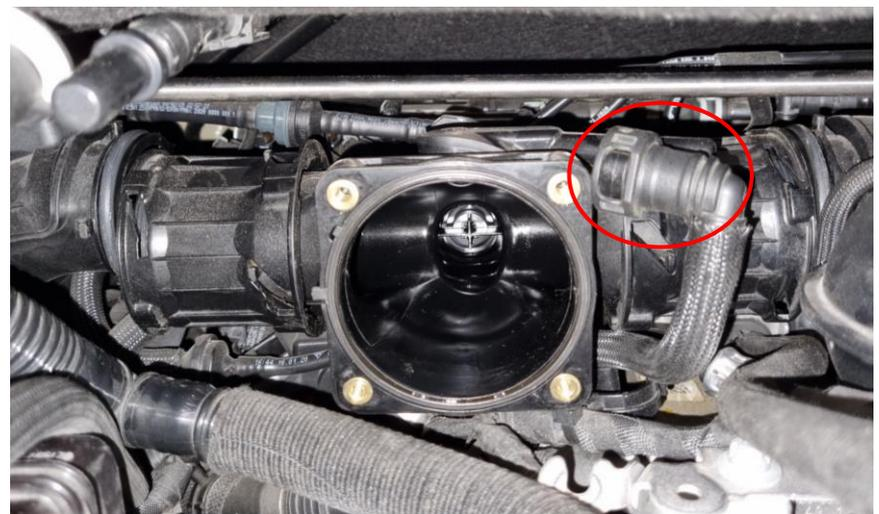
**29.** Loosen the square plastic tank and push aside to give more space. Also loosen other small ducts and parts that will give more room around the plenum.
