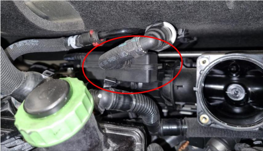
**30.** On both sides of the plenum screw the plastic sleeves towards the plenum. It helps to turn the entire plenum a little to loosen the sleeves.
