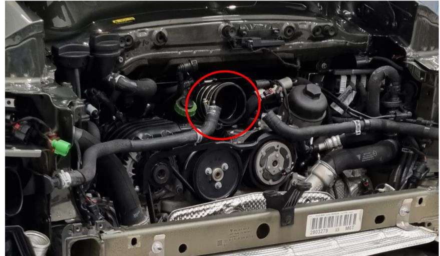
**27.** Remove the throttle body. Disconnect cable connector, 4x Torx E10 screws and 1x Hex 10mm nut.
