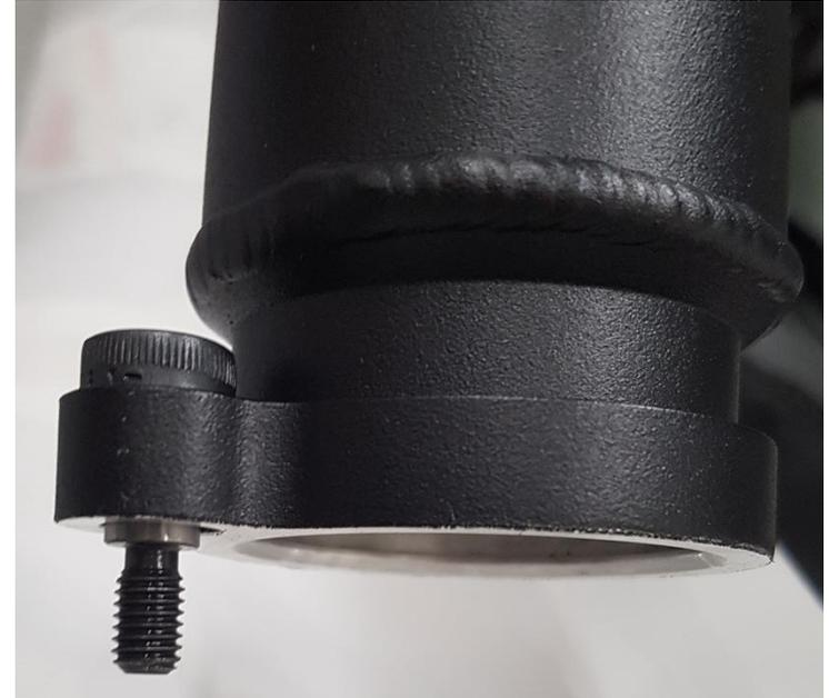
Because of the screw design, the pipe will not be fixed on the turbo and it should not be either.
