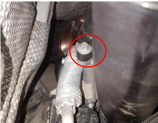
6. Disconnect the inlet pipe by removing 2x 6mm hose clamps, this makes it easier to access the E10 screw on the rear intercooler pipe.
