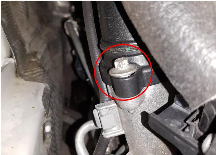
7. Remove 1x E10 screw that connects the rear intercooler Pipe to the turbo. This enables you to gently lift the pipe upwards and out of the car.
