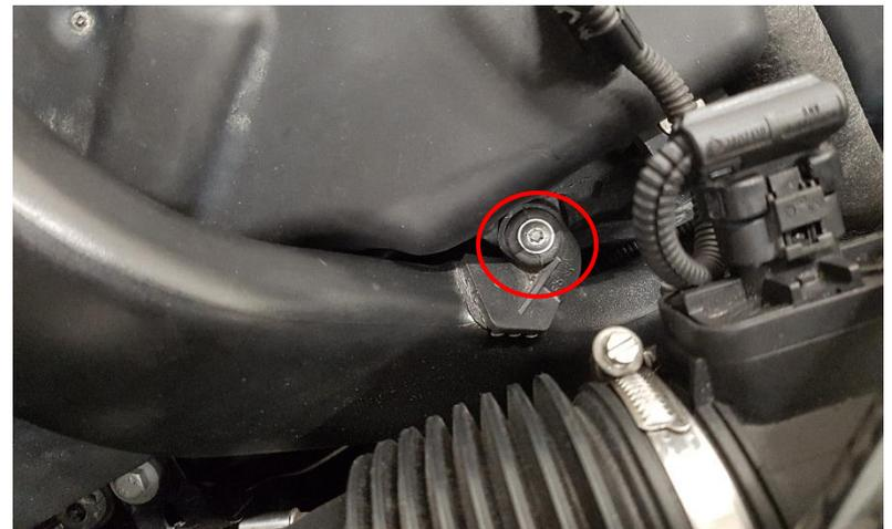
5. Remove 1x E10 screw that connects the front intercooler Pipe to the turbo. This enables you to gently lift the pipe upwards and out of the car.
