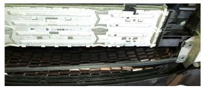
Remove 1x Torx T27 on each side of the intercooler then gently remove the intercooler from the car.
