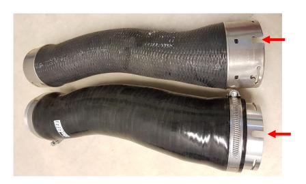
12. Install the pressure pipe into the car. It is most easy to do this from the upside. Reinstall clip, cable connector and small hose connection.
