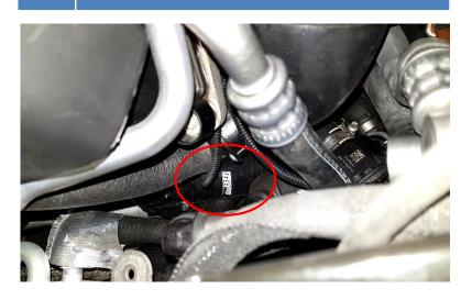
16. Now tighten the intercooler outlet hose hose clamp. Reinstall all other parts in reverse order.
