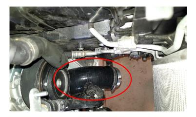
Now reinstall the intercooler. Before installing it put some lubrication on the connections to make the sealing slide on more easily.
