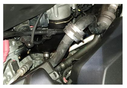
Push on the intercooler outlet hose onto the pressure pipe, do not tighten the hose clamp yet.
