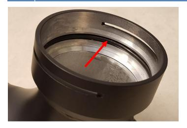
The OEM sealings and clips needs to be gently removed from the OEM hoses and installed into the do88 adapters.
