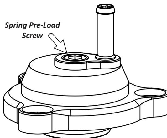
Increase the spring pre-load by 4 turns (clockwise) and repeat the above test, again listening to the sound and paying attention to the time it takes to get back to peak boost after a fast gearshift.
