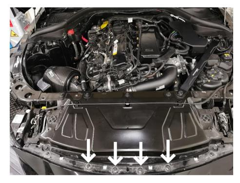
Remove the rubber seal and remove the 4 x 10mm hex screws holding the bumper cover.
