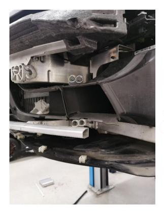
Remove the upper and lower screws holding the lower crash bar. 2 x E10 and 2 x 13mm hex screws on each side.
