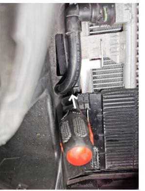
Now carefully loosen the oil line from the radiator support on both sides. Push the tab gently to release it.
