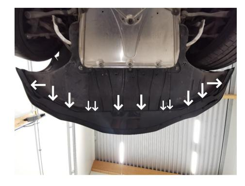
Remove the 12 x 8mm hex screws holding the bottom part of the bumper cover. Then preferably with the help of an assistant, remove the bumper. Start by pulling out the sides and disconnect the electrical connections on both sides, then pull the bumper forward to remove it from car.
