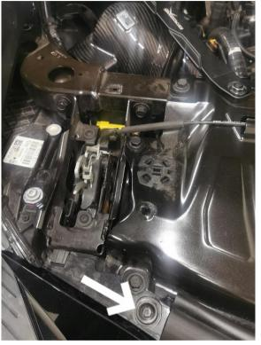
Remove the two plastic clips on each side holding the plastic panel over the hood latch.
