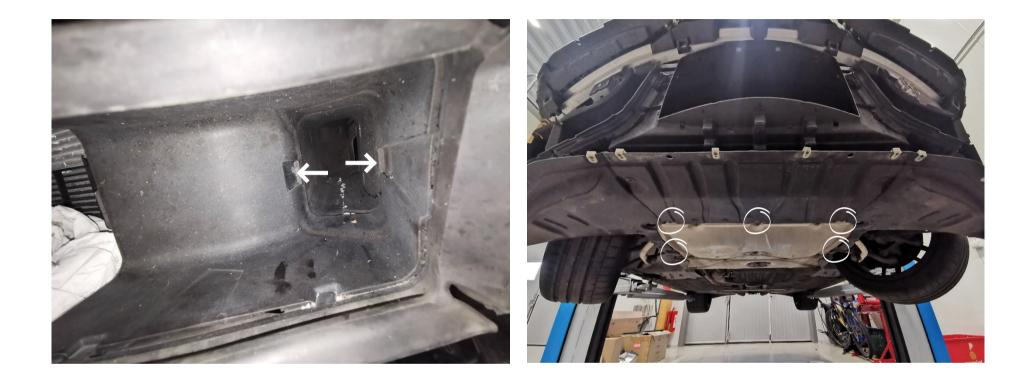
Remove the brake air duct by prying out the plastic clips and remove it in a backwards direction. Repeat on the other side.
