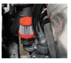
Step 6 Install the included air filter on the coupler and tighten the hose clamp.
