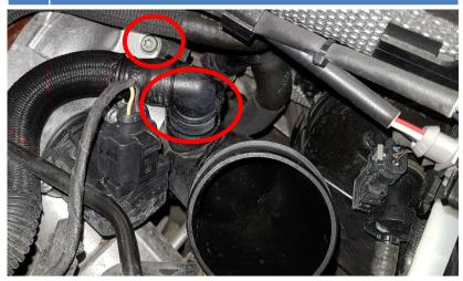
2. Remove the air filter box. Remove hose clamp, vacuum hose, SAI-connection (if your car has it). Then pull the air filter box upwards (it can sit quite hard in its rubber bushings).
