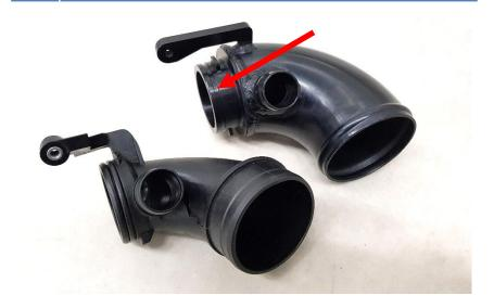
**5.** Install the do88 inlet pipe in the car. Use the included silicone hose and hose clamps between the inlet pipe and air filter box. Reinstall all other parts in reverse order.
