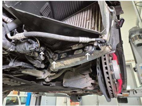
Remove the lower intercooler hoses on both sides by loosening the 2x hose clamps.
