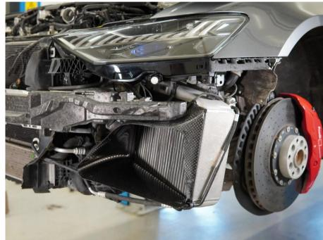
Install both carbon fiber air guides by gently sliding them in from the side. Fasten them with the included M5x8 mm Allen screws, but do not fully tighten them yet.
