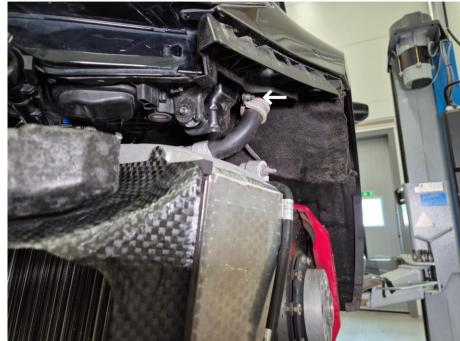
Reinstall both lower intercooler brackets. While tightening the 13 mm hex screw, gently lift the intercooler slightly upward to ensure proper alignment / clearance.
