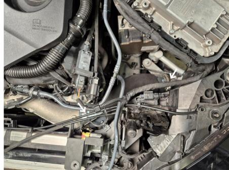
Remove the upper intercooler hoses on both sides by loosening the 2x hose clamps.
