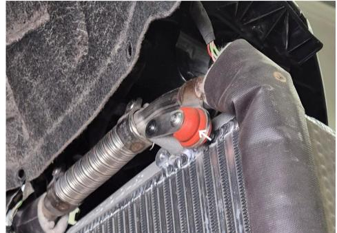
If your vehicle is equipped with a parking heater, install the supplied brackets using the included M5x12 mm Allen screws. Ensure the small hole faces the intercooler. The brackets is shown with arrows in the photo.
