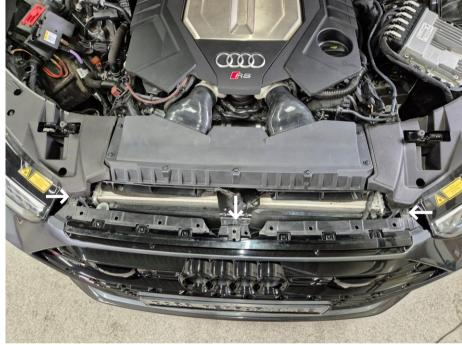
Remove the front bumper cover, the 9x plastic clips, and the hood release handle (press the plastic tab inward and pull it straight up).
