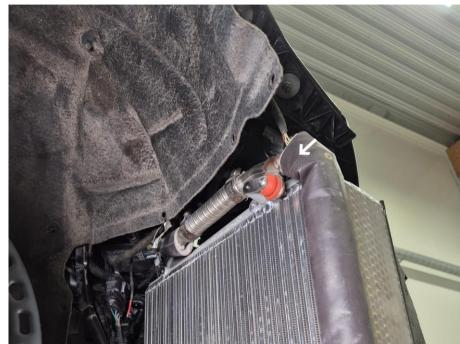
Detach the wiring harness clips from the top of each intercooler tank on both sides. Then remove the front intercooler air ducts by releasing the plastic tabs (marked with arrow in the photo) and pulling them off.
