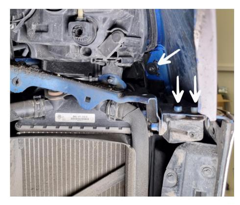
From the wheel arch, remove 3x Torx T30 that holds the bumper cover, do this on both sides of the car.
