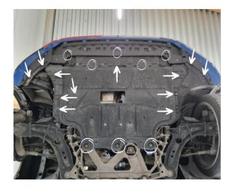
Remove 6x Torx T45 and 11x Torx T25. Use a flat head screwdriver to separate the plastic tabs and remove the plastic cover underneath the car.
