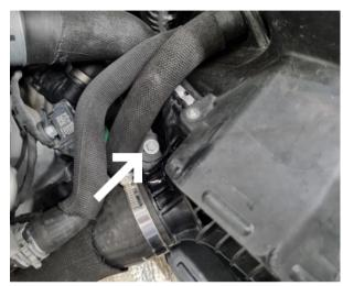
Step 17 Remove 1x Hex 10mm screws on each side of the intercooler.
