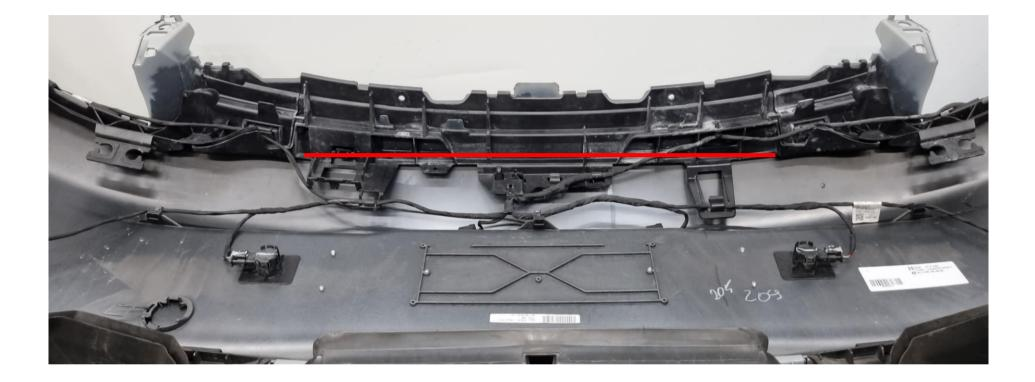
Inside the upper parts of the rear bumper disconnect the cables from their original position and relocate them behind the plastic tabs on the marked area on the photo below. Fasten the cables with the included zip-ties.
