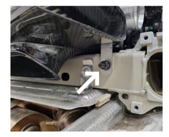
Gently lift the intercooler package into the car, start with the throttle body hose, then into the center rubber grommets.
