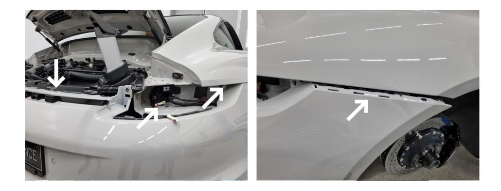
On both sides remove 2x Torx T30 and disconnect 1x cable connector marked on photo.
