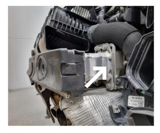
Step 15 Remove the crash bar. 4x Hex 13mm on each side.
