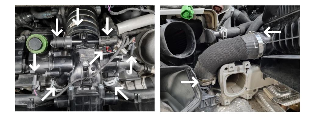
Disconnect 3x cable connector / 1x cable holder / 2 x vacuum lines / 2x rubber hoses to the BOV:s. Also loosen the hose clamp to the throttle body hose.
