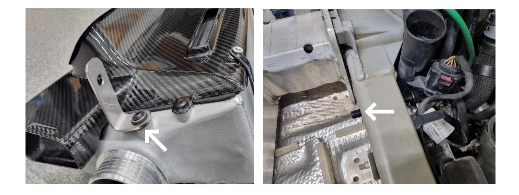
Underneath each intercooler inlet tank install the included brackets.
