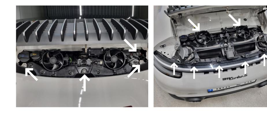
Remove 3x Torx T30 screws and disconnect the brake light cable connector. Then gently pull this panel backwards and lift it straight up. Be careful not to damage the paint around the spoiler mechanism.
