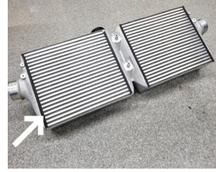
On both sides of the intercooler assembly remove the small air channels. 3x Hex 10mm.
