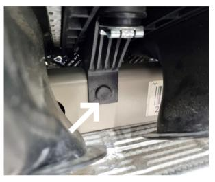
Step 16 Pull out the plastic pin with suitable pliers.
