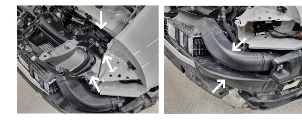
Remove the spoiler mechanism. 4x Torx T45 and 2x cable connectors.
