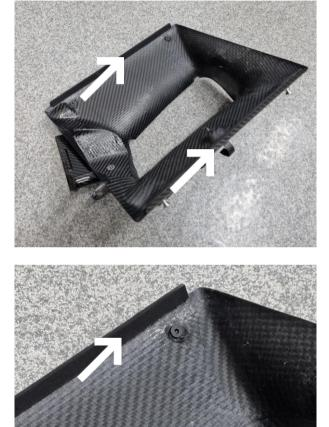
On all 4 carbon fiber air guides fasten the included 3x10mm adhesive foam strip on the inside of the lips
