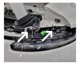
Remove the outer rear light. 2x Torx T30. Disconnect the cable connector. Do this on both sides.
