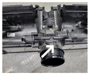
On both sides remove the intercooler brackets, pull out the plastic pin with suitable pliers.
