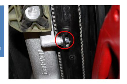
The lower right hand side plastic radiator bracket may need to be trimmed, to give clearance for the condenser pipes.
