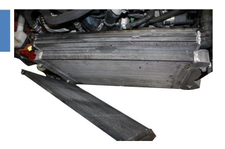
Remove the stock intercooler brackets and install them in same location on the do88 performance intercooler.
