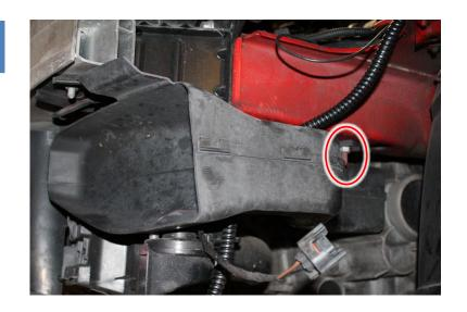
12. Remove 8x Hex 16mm screws for the two radiator bulkhead main brackets.
