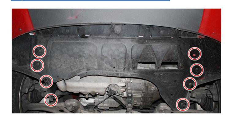
**3.** Remove 4x Torx T25 in each inner fender.
