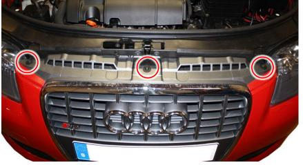
7. With help from a friend bend out the bumper on each side and pull it forward about 20cm and hold it in this position.
