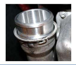
132. Install the do88 right hand side intercooler hose. Tighten it with the included hose clamps. Make sure the hose is orientated without any kinks.
