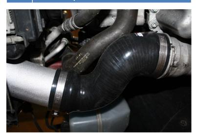
133. Install the do88 left hand side intercooler hose. Tighten it with the included hose clamps. Make sure the hose is orientated without any kinks.
