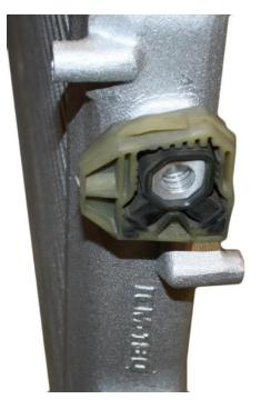
23. Install the do88 performance intercooler between the radiator and condenser. Connect the intercooler to the radiator with four of the included M6 x 15mm screws.
