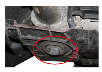
With a friends help, remove the two included M10 x 120mm from both sides of the radiator bulkhead (these are the ones from step 12 in this guide).
