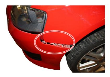
8. On cars equipped with headlight washers, clamp the headlight washer hose with a suitable tool as shown on the photo.
