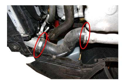
Find a support in proper height that you can put underneath the radiator/intercooler/condenser assembly.
