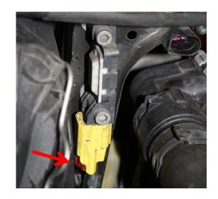
Disconnect the fan wiring connector from below the car. Then disconnect the remaining connectors in this wiring harness such as fog light and ambient temperature sensor.
