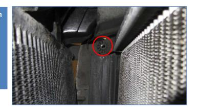
17. Intercooler installed together with AC condenser, engine oil cooler and power steering pipe.
