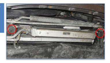
Loosen the engine oil cooler that are attached to the intercooler with 2 pcs 10mm hex screws.
