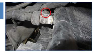
Separate the condenser from the intercooler by sliding it downwards from the intercooler.
