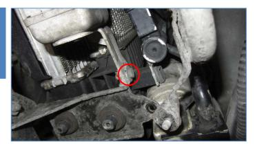
Remove inlet pipe from air filter box be removing the hose clamp using a 7mm hose clamp screwdriver or 7mm hex socket. Then pull apart inlet pipe from air box.
