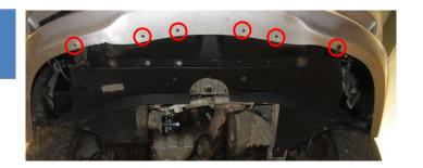
2. Remove the 1pcs screw on each side of vehicle that holds the bumper to the inner fender.
