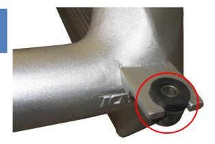
Hold the intercooler in place so the bushings align with the screw holes for the intercooler without installing the screws.
