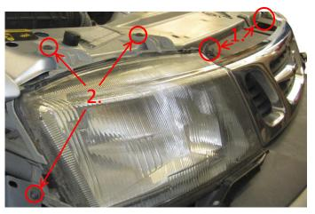
7. If vehicle are equipped with headlight vipers, first remove the washer hose from the viper blade arm and then remove them by folding up the plastic cover (1.), removing the 8mm hex nut (2.) located underneath and then wiggle it a bit at the same time as you pull it of the axle.
