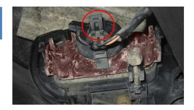
5. Remove front indicator lights by removing the 1 screw that attaches it to the headlight from the top. Then pull the indicator light forwards and remove the electrical connection.
