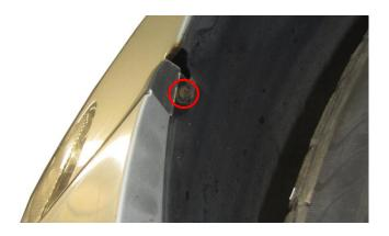
Remove the 1pc screw on each side that attaches the plastic radiator protection to the inner fenders.
