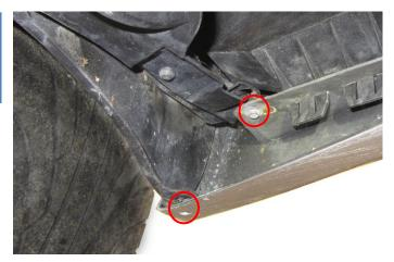
4. Disconnect the fog light electrical connectors from underneath by prying out the retainer clip and pulling it downwards from the lamp connector.
