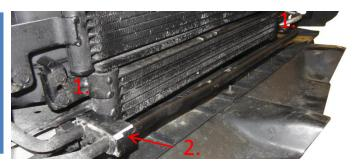
13. Install the intercooler with the 2pcs 10mm hex screws.
