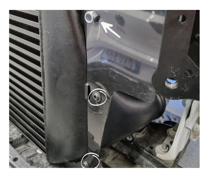
Install the included plastic airguide with the 2x included m6x12 black Allen screw and 1x m8 nut (with nylon lock) so the m8 nut (without nylon lock) is located behind the airguide as a spacer. Do this on both sides of the car.
