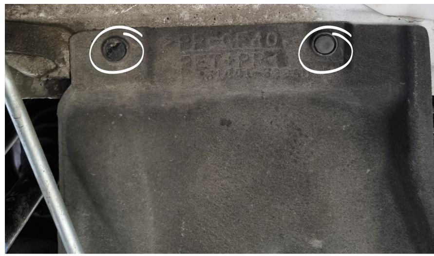
Inside the right-side wheel arch remove 2x plastic clips with a small flathead Remove 2x 10mm hex screws holding the OE charge pipe. screwdriver. Loosen hose clamp, 1x 10mm hex screw.
