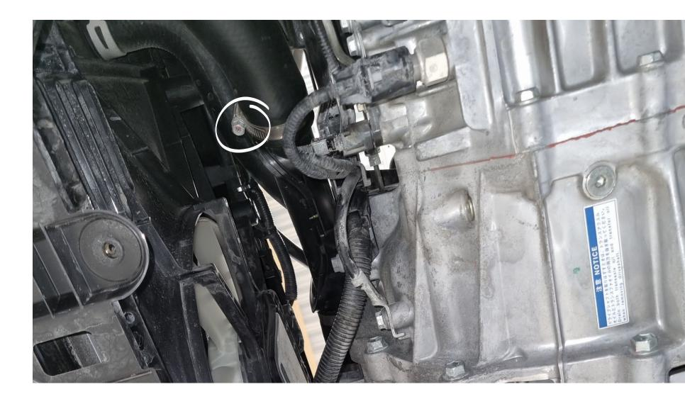
Loosen hose clamps, 2x 10mm hex screws and remove the intercooler outlet hose from the car.
