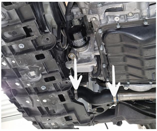
Loosen hose clamp, 1x 10mm hex screw and remove the OE turbo outlet hose from the car. Step 7
