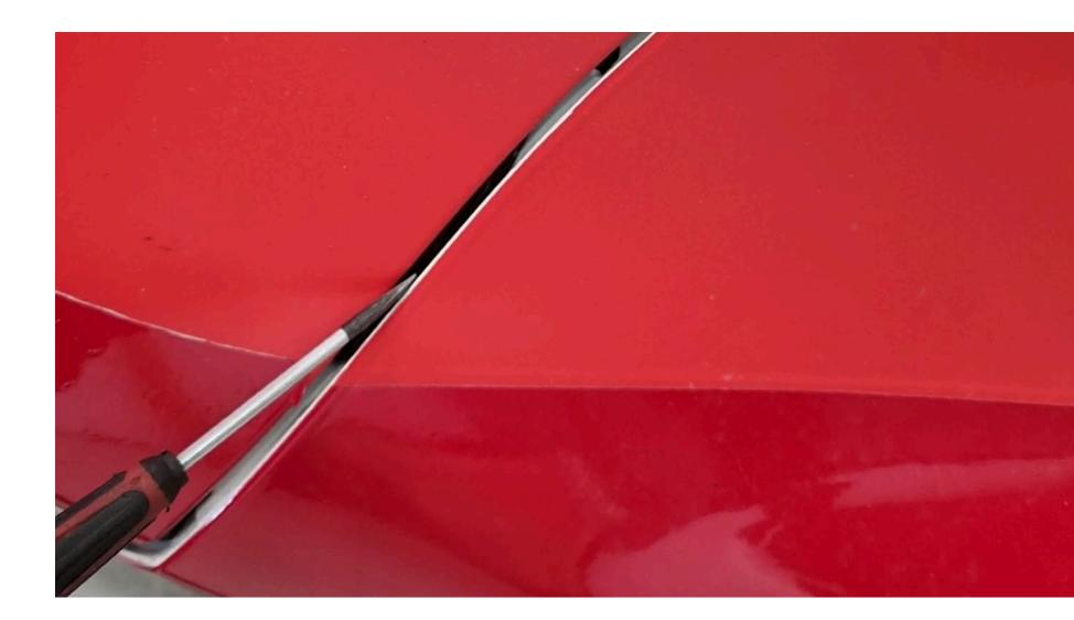
Seperate the front bumper from the front fender with a small flathead screwdriver and gently rotate the screwdriver and pull the front bumper towards yourself.
