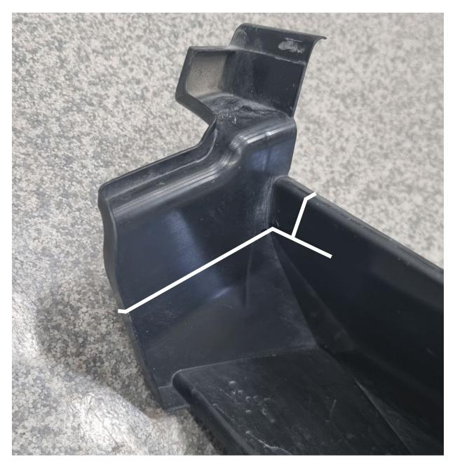
Cut the upper plastic airguide as shown on picture. Re-install all other parts in reversed order.
