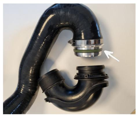
Install the included joiner on the hose and re-use the OEM O-ring from the intercooler pipe and install the do88 hose in the car.
