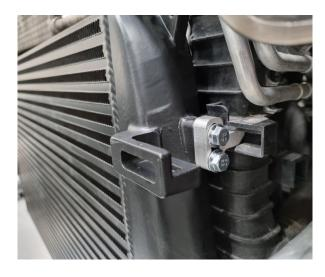
Remove clamps with a 6mm hex screwdriver and disconnect the intercooler pipes on both sides.
