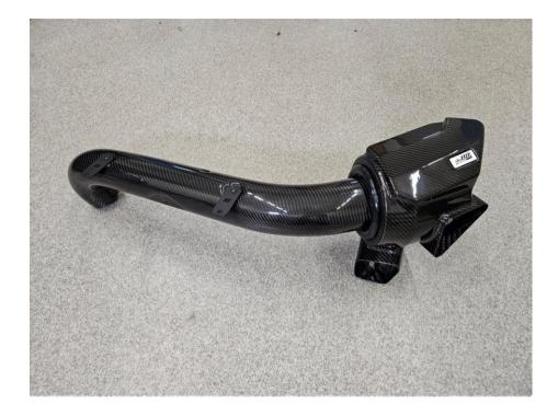
Mount the large bracket with 3 holes to the left air filter housing using three included M6 screws. Do not tighten the screws yet.
