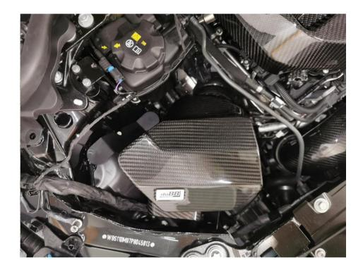
Assemble the intake pipe and filer with the air filter housing. Then install them in the car starting with seating the housing in the OEM rubber bushings and then mount the silicone hose to the rear turbo inlet and clocking the filter assembly before tightening the hose clamp.
