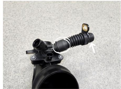
Remove the front turbo inlet pipe by removing the two Torx E8 screws holding it to the turbo.
