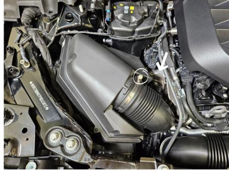
Remove the front V-shaped strut tower brace by removing the 13mm hex screw in the front. Remove one plastic retaining clip to reveal and remove two 15mm nuts, repeat on the other side.
