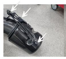
Check the rotation of this metal ring towards the air filter housing by lining up the 3 holes towards the holes in the carbon fiber air filter box. Then install the included rubber sealing strip on the metal ring with the edges on the rubber sealing pointing to the bottom of the air filter box.
