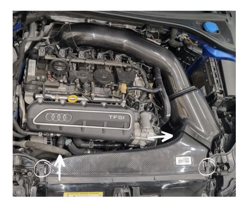
Install the carbon fiber air duct by sliding the opening with the self-adhesive rubber sealing into the air filter box and gently push the AC-hose towards the engine then slide the front air duct into place, secure it with the 2x included M5x12 black Allen screws. Gently apply some pressure with your hands on the bracket (not on the carbon fiber air filter housing) under the air filter box to make the rubber bushings sit into place.
