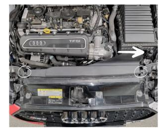
Remove the engine cover, grab the corners of the engine cover and gently lift it upwards.
