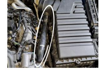
Install the included O-ring on the machined adapter, lube the o-ring then install the machined adapter into the charge pipe.
