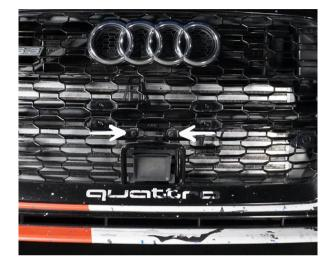
Re-install the upper part that was separated from the lower in the previous step back into the front bumper and secure with 11pcs Torx T25 screws and re-connect the parking sensors.
